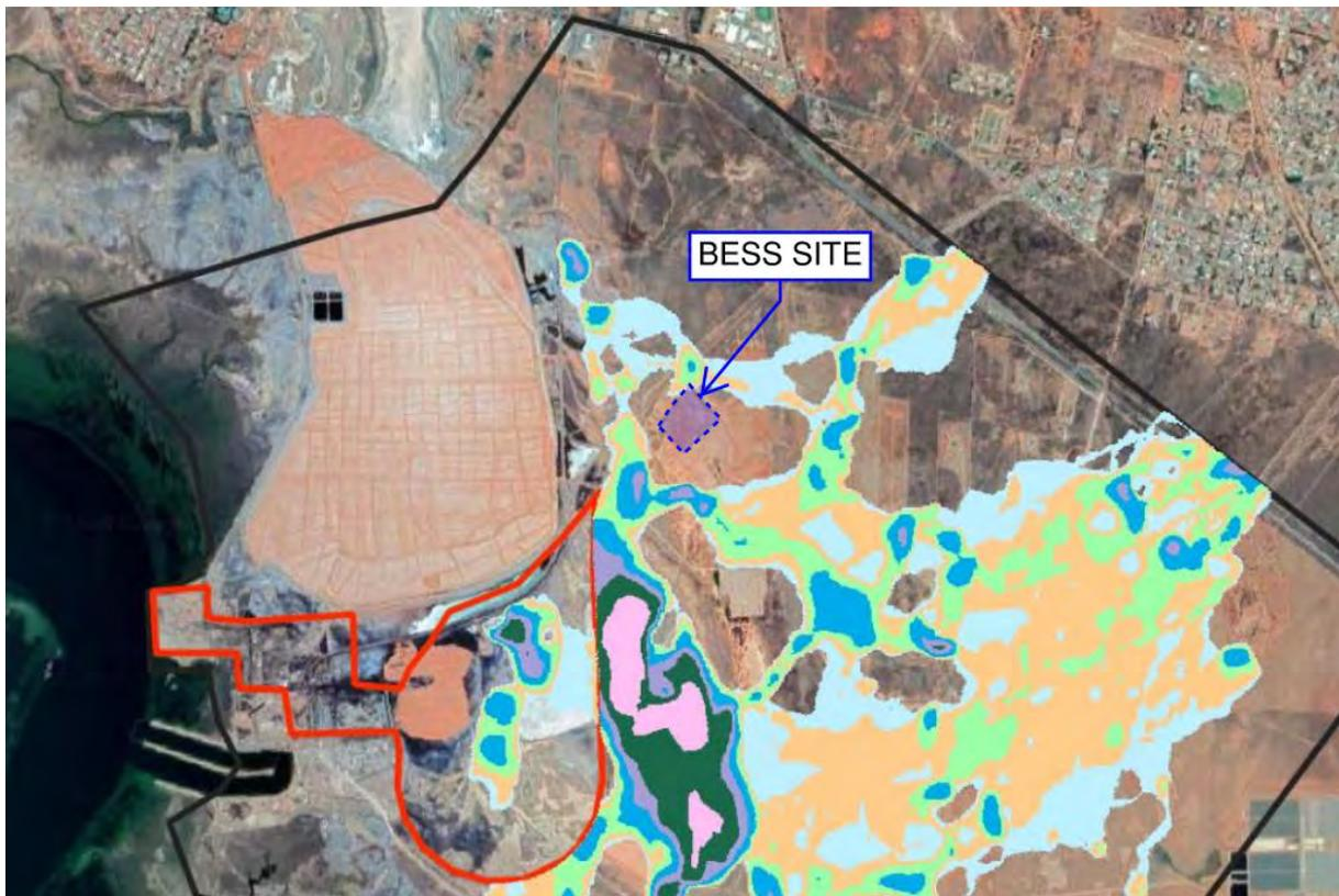
**Figure 2: Water Technology 1% AEP Flood Inundation Map, Site Outline in Blue**
