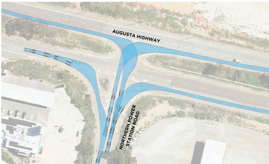
*Figure 2 - PBS Level 3A Vehicle Turns at the Augusta Highway/Northern Power Station Road intersection*
